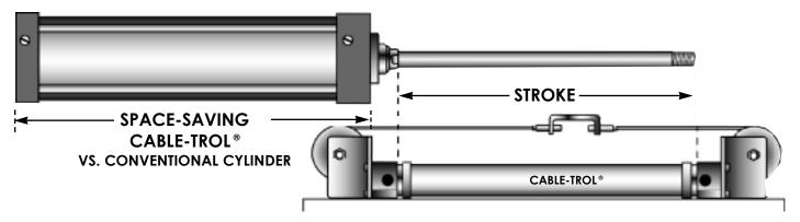
CABLE-TROL® cylinders provide the same stroke as conventional cylinders with about 50% SPACE SAVINGS. As the piston is pushed in one direction, the load is pulled in
